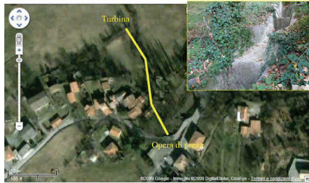
Fig. 1. Study site. The intake is located at 360 m aswl and the turbine at 334 m aswl
